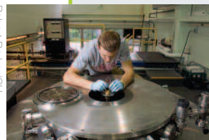
Graduate student David Chalenski inserts an array into the COBRA pulsed power generator.
